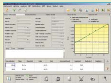
Patient Sample Report, containing a factor inhibitor. The Parallelism curve (prediluted patient sample) intersects with the calibration curve.
